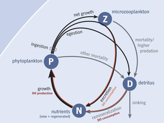
The biogeochemical model consists of a four-compartment nitrogen budget plus dissolved oxygen. It has been kept very simple to minimize the number of components that cannot be compared with observations.
