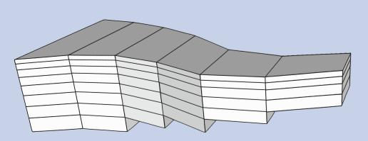
Tonicella is a finite-volume model with a fixed cartesian grid in the along-channel (x) and vertical (z) directions. Width is allowed to vary in the x direction. At each timestep, velocity and vertical diffusivity are calculated, tracers are advected and mixed, and biogeochemical transformations are calculated
